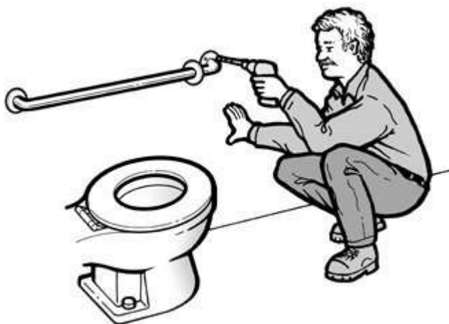
Grab Bar Installation
